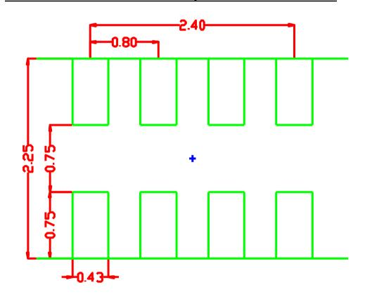
Superposition of terminal sharpes of RA1632 and RM3216
