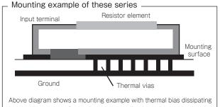
Above diagram shows a mounting example with thermal bias dissipating heat to the ground. Depending on the application, a heat sink might be needed closely contacting to the bottom of the product.
